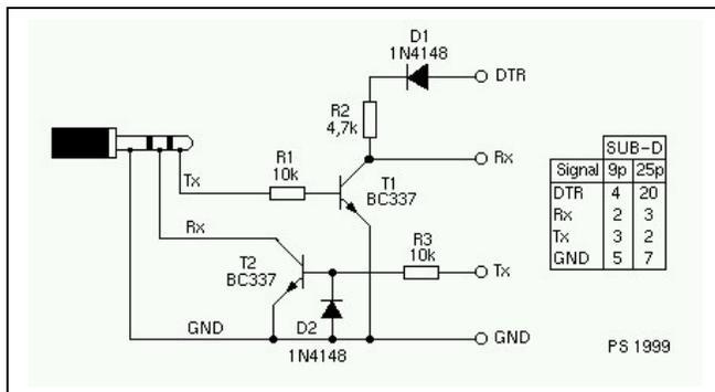
2.5 mm stereo plug from Casio connected to a PC D9 female plug.
